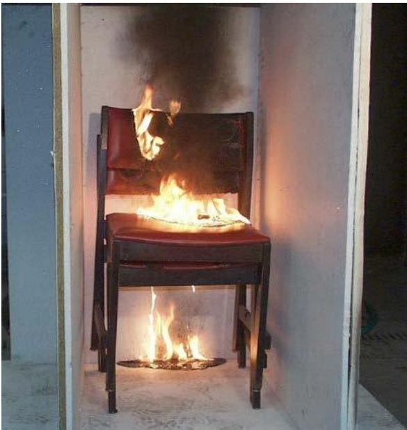
Photo 3. Ignition with plastic boxes and intense Gorenje after 15 minutes
